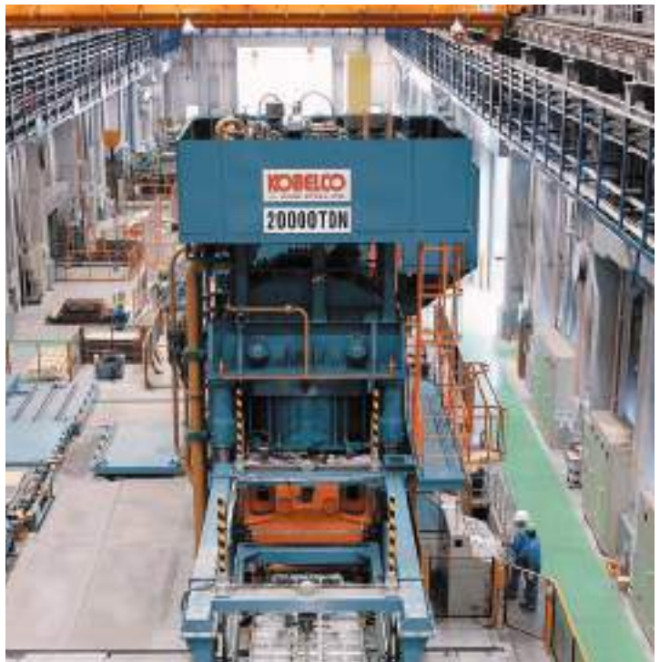
Fully-automated 20,000 ton press
