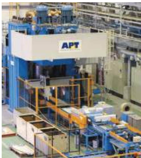
High-speed, automated 4,000 ton press
